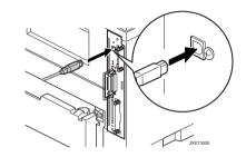
Attach the other end of the interface cable to the USB interface connector of the computer or the USB Hub. Secure the cable.
